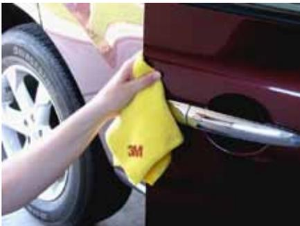
3. Always check part position, shape and size before applying. The Door Edge film is rounded on the ends; if desired it can be cut straight.
