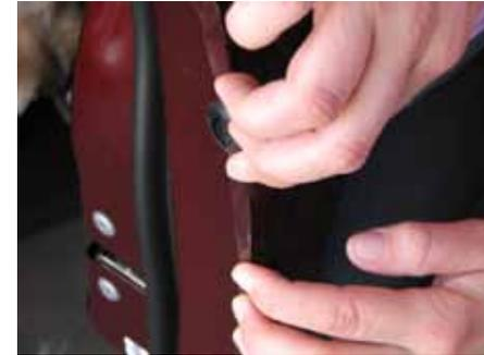
8. After starting to secure the edge, continue to fold the film around to the back of the door edge over the entire length of the door.
