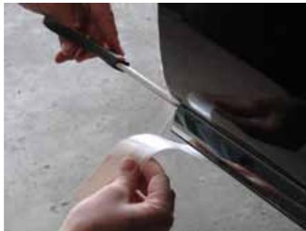
7. Begin pressing the film around the edge of the door over the entire length of the door, but not all the way to the back side yet. This will help to prevent air bubbles.
